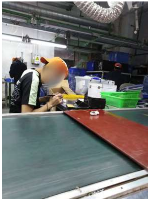
(Soldering position without an exhaust fan)
