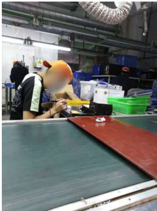
(Soldering position without an exhaust fan)
