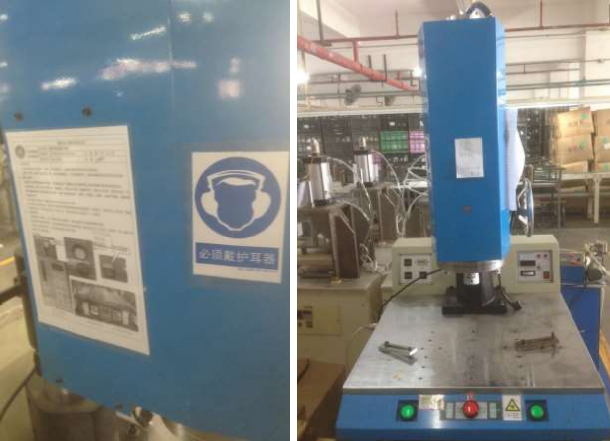
(Ultrasound machine in the workshop with a notice that hearing protection must be worn)
