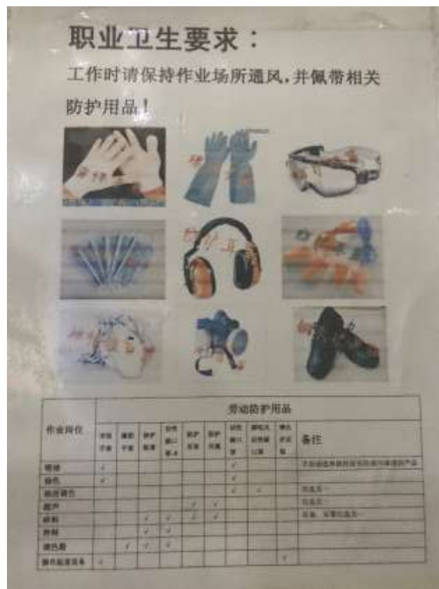
The flyer above lists the personal protection equipment as required for different positions in the workshops
