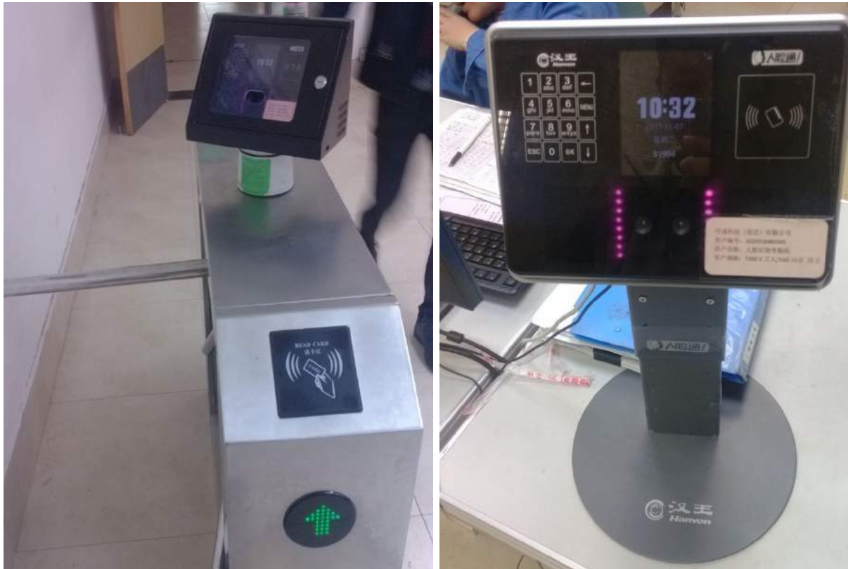
(Left: Turnstile with card reader and facial recognition machine; Right: Facial recognition machine)
