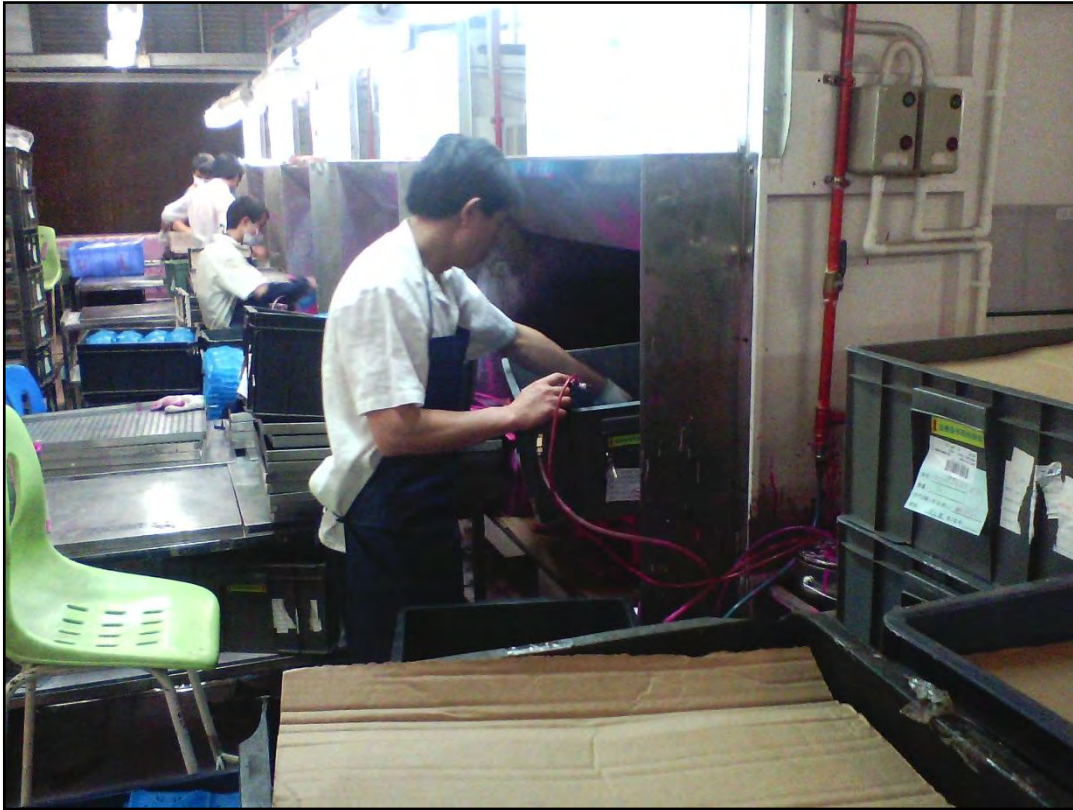
Paint spraying worker not wearing mask while working
